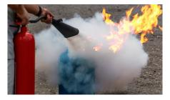
**Where should CO2 be used?** Gas extinguishers are the best solution for preserving delicate equipment that could be damaged by water or powder based units. They are also tested and suitable for use on Class B flammable liquid fires.
